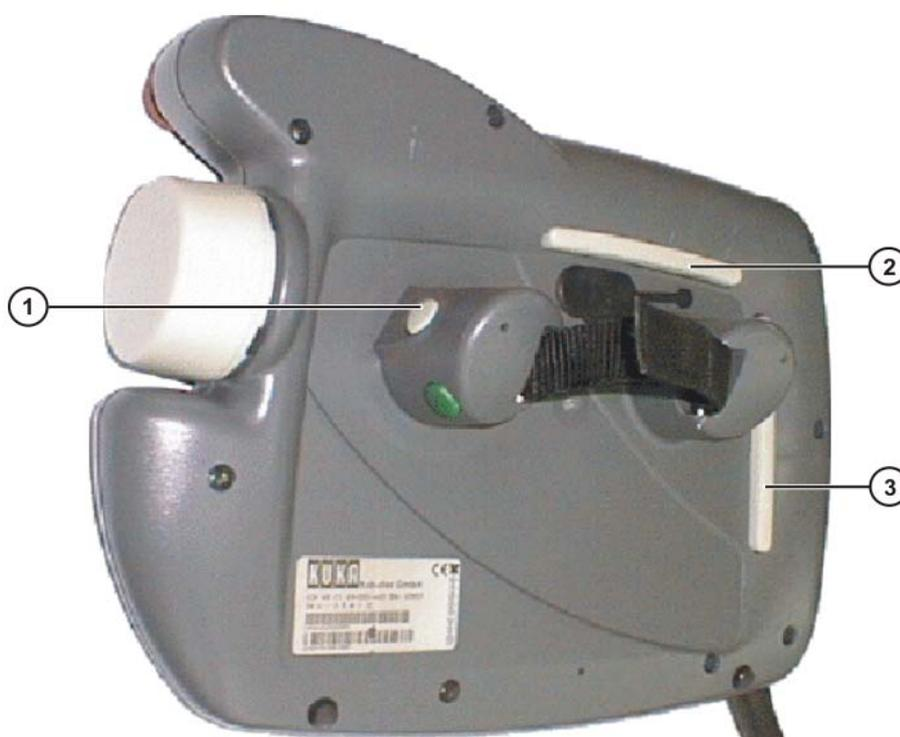
**Fig. 3-5: Enabling switches on the KCP**
